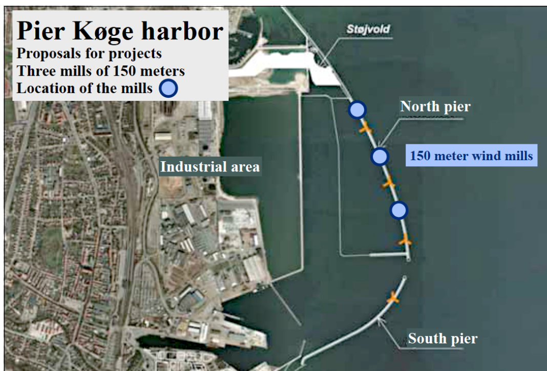
Figure 2. The third wind mill project: Coastal wind turbines on the new pier at Køge Harbor.
